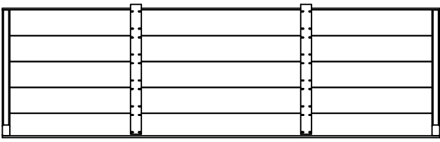
(2) RP2 - DACHPLATTE - W2A01678 1 3/4"x16 1/4"x53 3/4" (45x412x1366)
